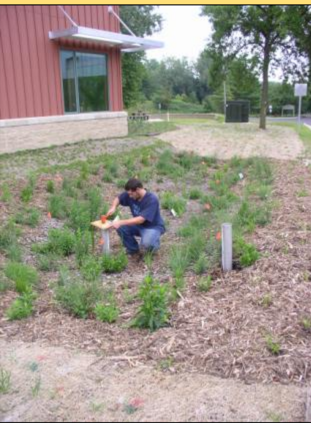
Synthetic Runoff Testing of a rain garden in Little Canada, MN (Photo courtesy B. Asleson & R. Nestingen)
