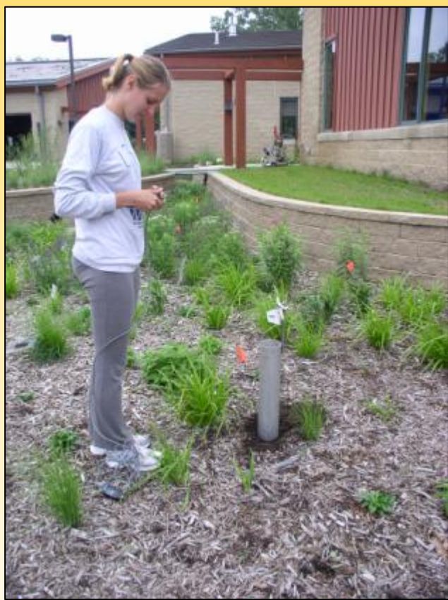
Synthetic Runoff Testing of a rain garden in Little Canada, MN (Photo courtesy B. Asleson & R. Nestingen)
